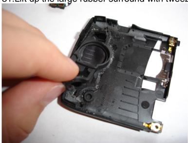
32. Lift up the mesh below with tweezers and transfer it to the new aerial cover.
