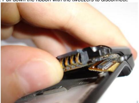
23. Push the bottom sideways away from the top this should unclip the Aerial Cover from the lower & mic housing. If not use the Mobile Phone Opening tool around the edge and flip up the edges.
