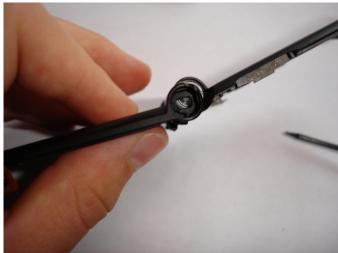
42. From the outside push out the flicker using a screwdriver. Then pull it out from the other side. Make sure you remove the flipper and its black housing.
