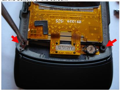
9. Lift the small battery and ribbon off of the inner screen housing. Use tweezers to gently ease it up.
