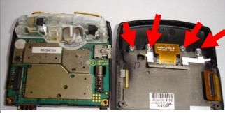
24. You now need to unscrew the 4 screws holding the lower cover on. Use the T5 screwdriver.
