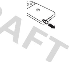
2 Press down the release latch, then slide the battery door away from the camera lens and remove it from the phone.
