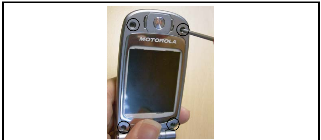
Figure 9. Removing the 4 Screws
