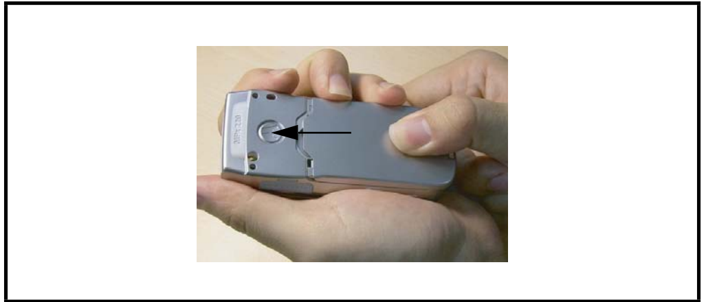
Figure 5. Replacing the Battery Door
