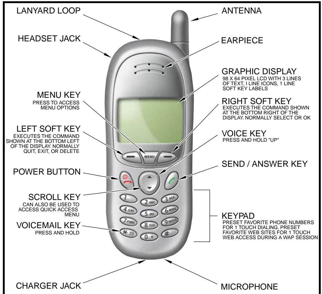
Figure 1. PF C25 Controls and indicators locations
