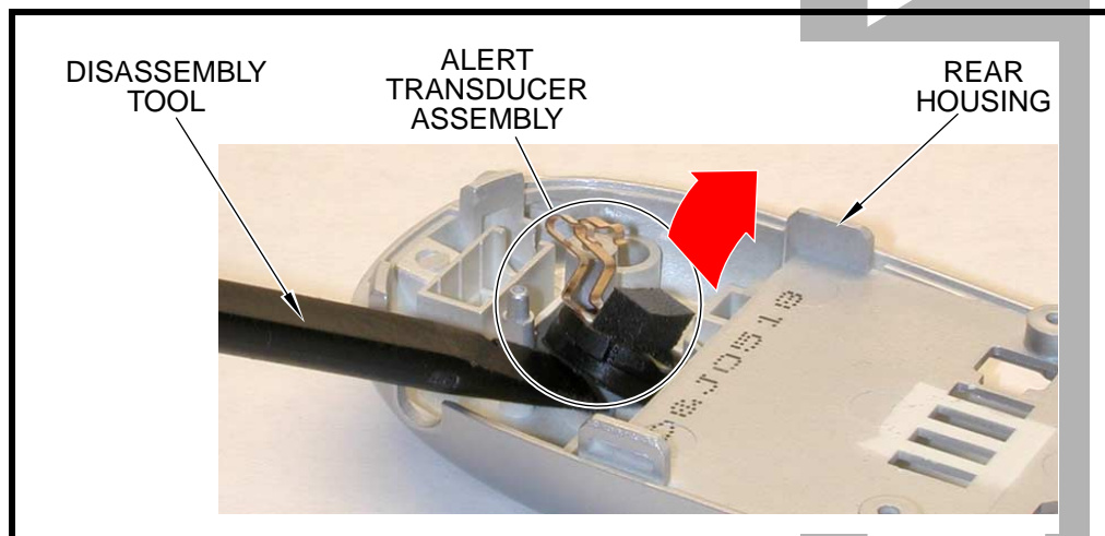
Figure 13. Removing the alert transducer assembly
