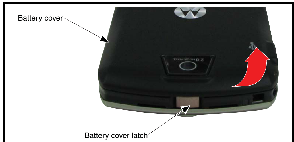
Figure 3. Removing the Battery Cover
