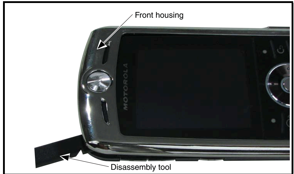
Figure 14. Releasing the Front Housing Catches
