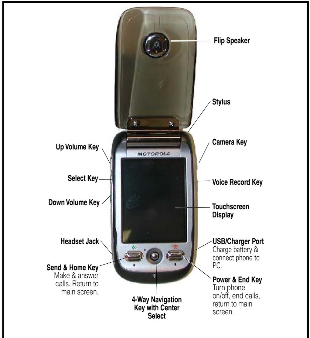
Figure 1. Telephone Controls and Indicators Locations (Front)
