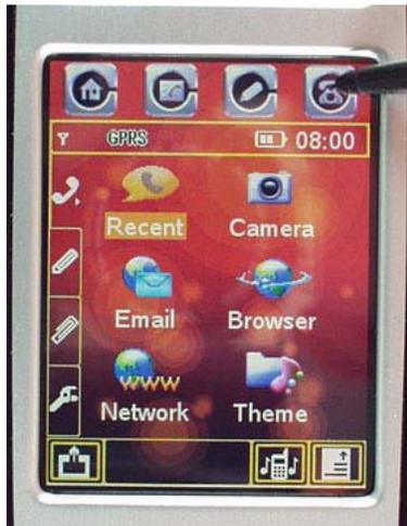
8. On the dial mode screen, tap and hold the # key for 3 seconds to enter the Test Menu.
