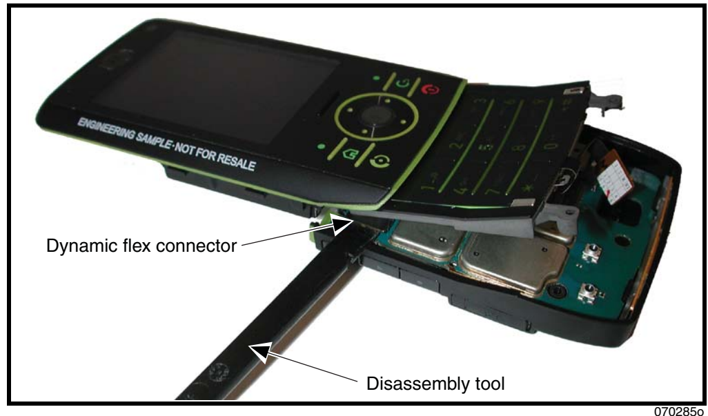
Figure 11. Removing the Dynamic Flex Connector
