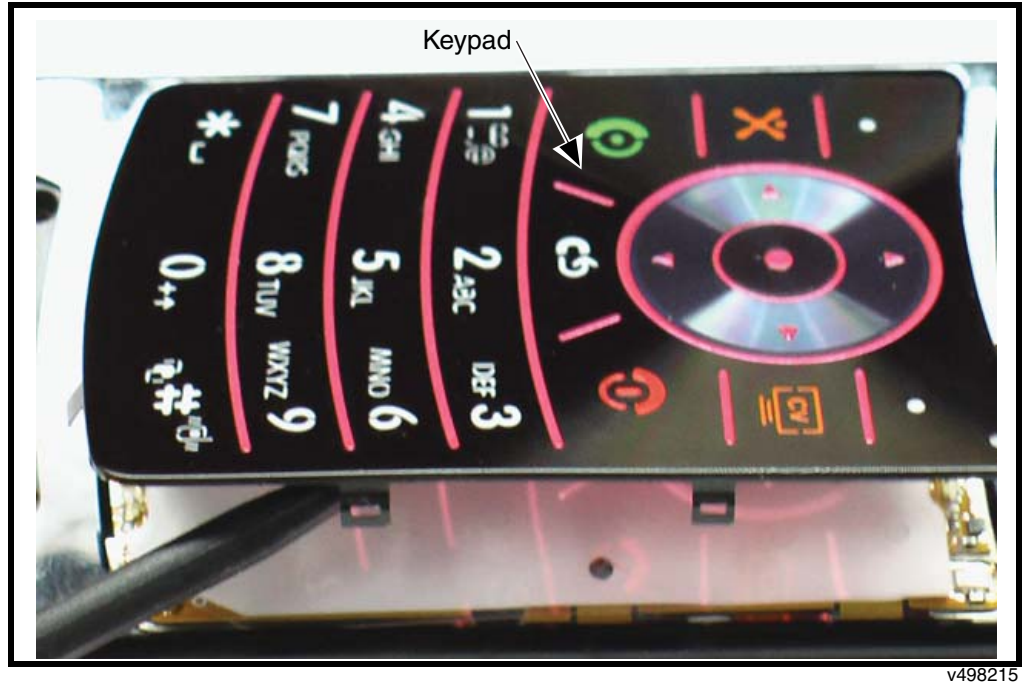
Figure 20. Placing the Keypad into the Front Housing
