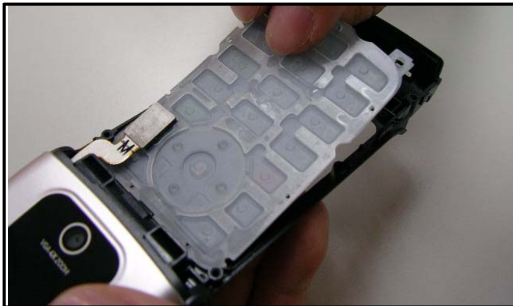
Figure 25. Removing the keypad
