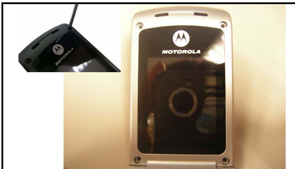
Figure 28. Removing the four T5 screws
