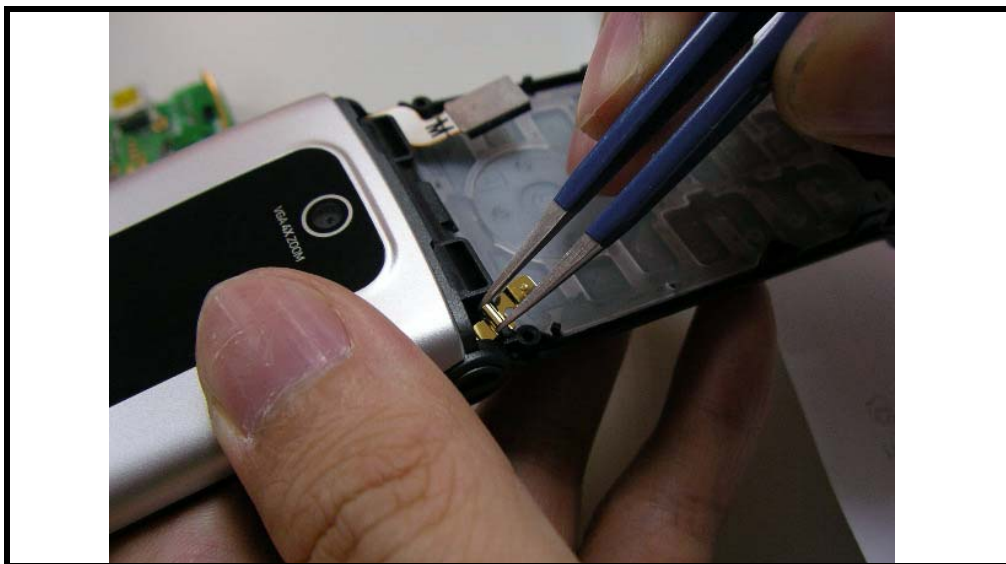
Figure 24. Prying the spring
