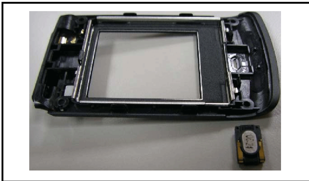
Figure 41. Removing the receiver
