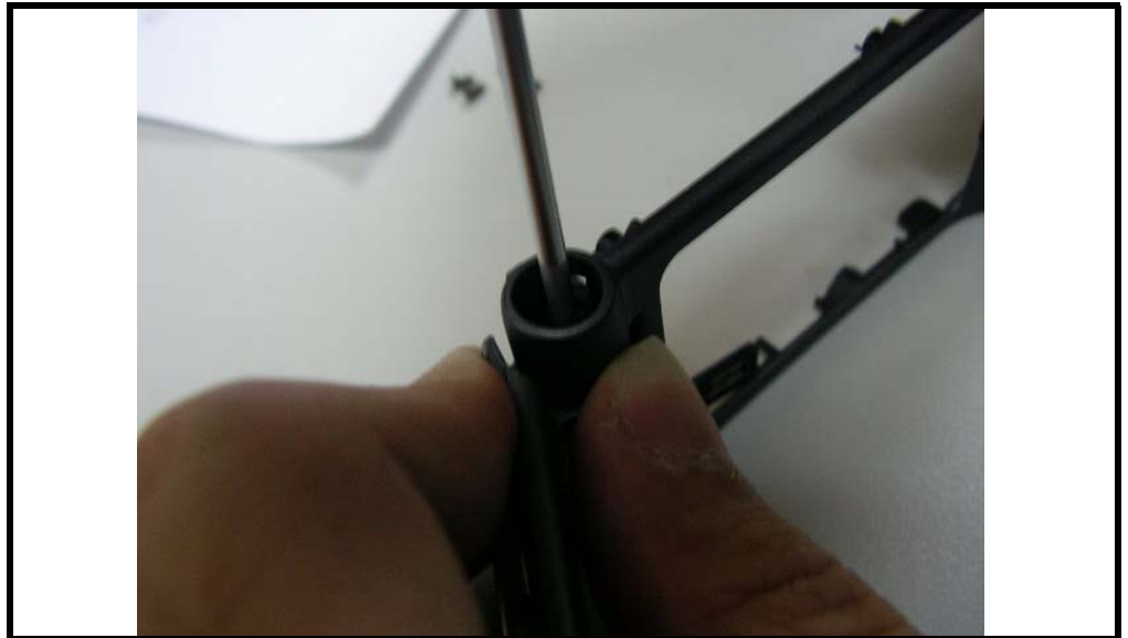
Figure 33. Exerting pressure on the clamshell
