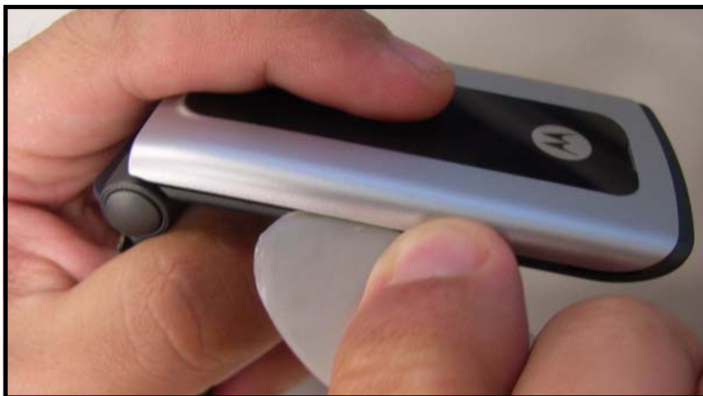
Figure 29. Disconnecting the two halves
