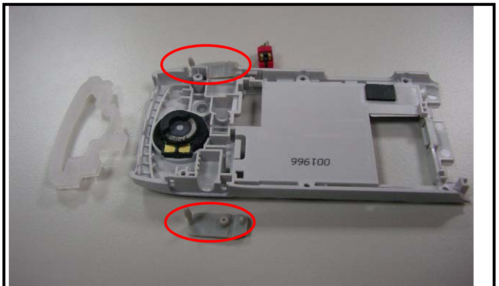
Figure 16. Removing the rubber pad
