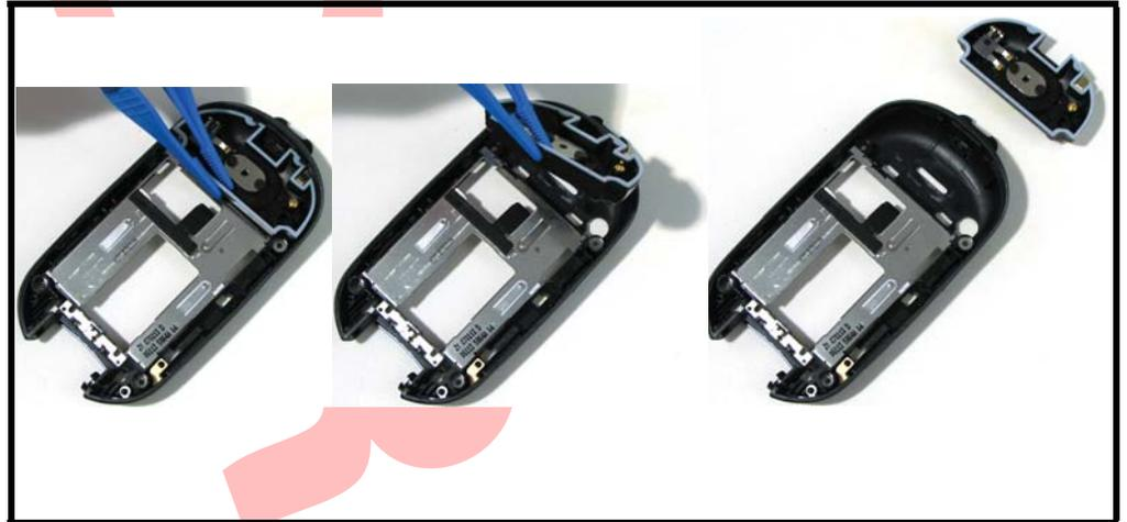
**Figure 19. Removing the Antenna from the Housing**
