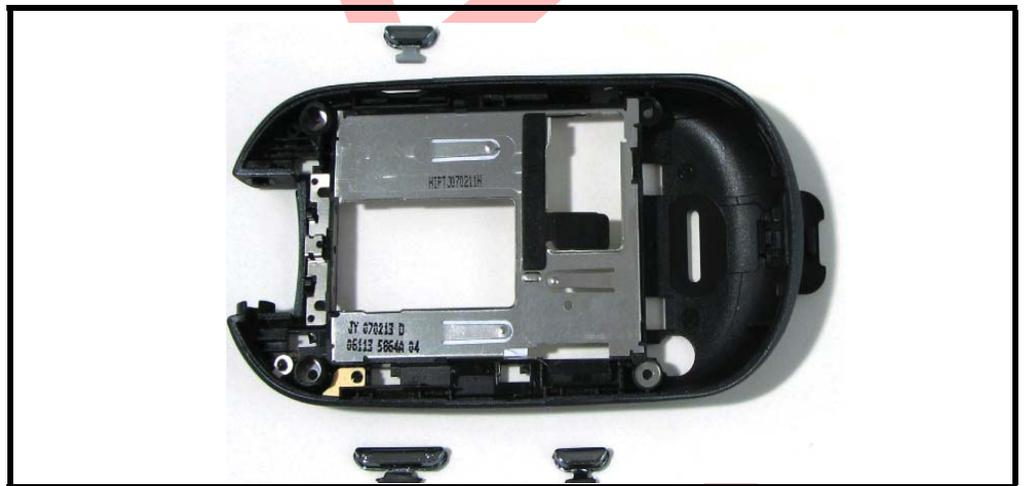
**Figure 20. Removing the Front Housing Assembly**
