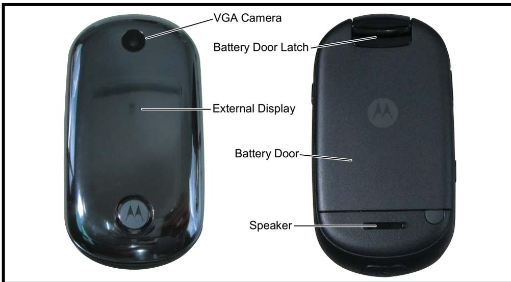
Figure 2. Telephone Controls, indicators, and I/O Connections (Flip Closed)
