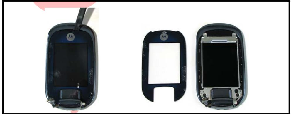
**Figure 10. Removing the Main Lens to Expose Housing Screws**
