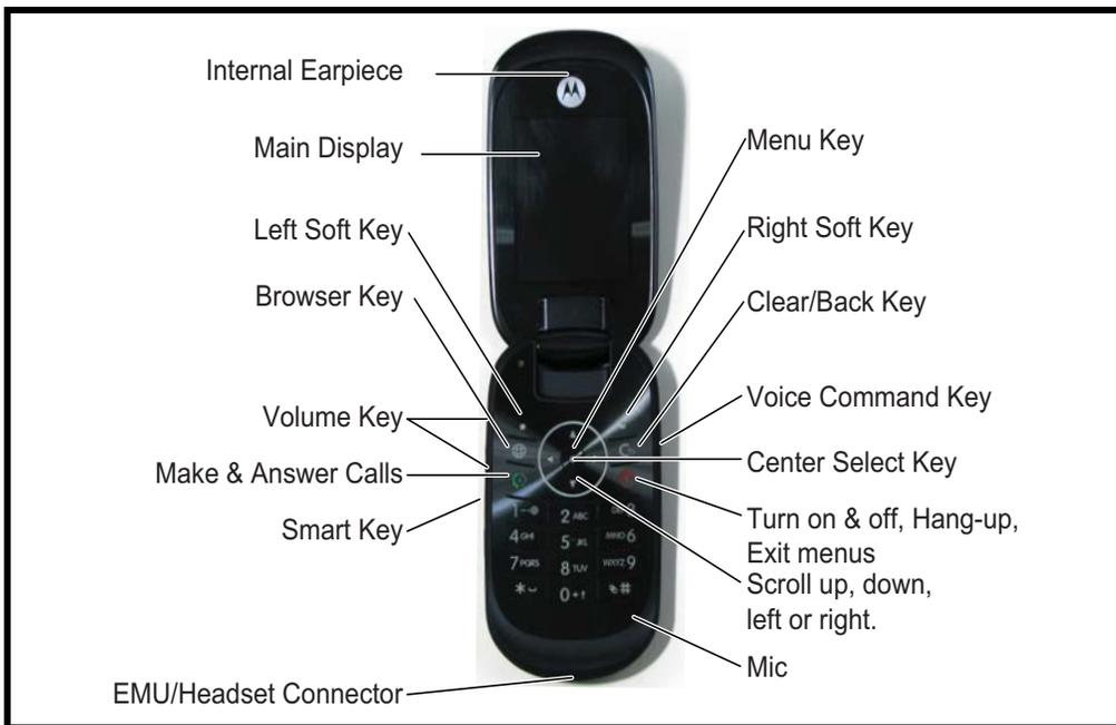
Figure 1. Telephone Controls, indicators, and I/O Connections (Flip Open)
