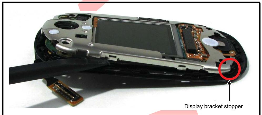
Figure 15. Removing the Display Bracket Assembly
