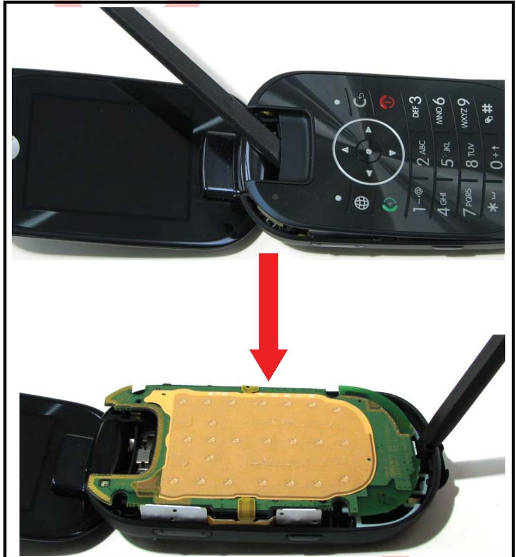
**Figure 5. Removing the Keypad to Access the Xcvr Assembly**
