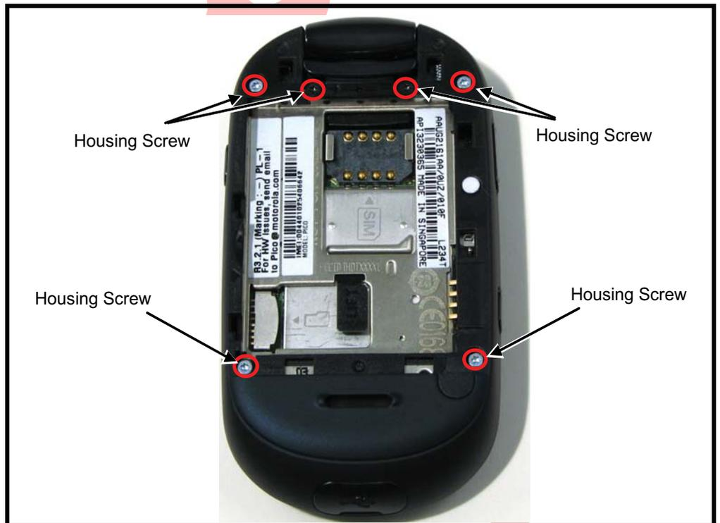
**Figure 4. Removing the Rear Housing Screws**
