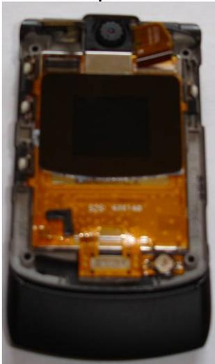
53. CAREFULLY connect the camera ribbon up, remember to lock it down. Now connect the main left ribbon back up.
