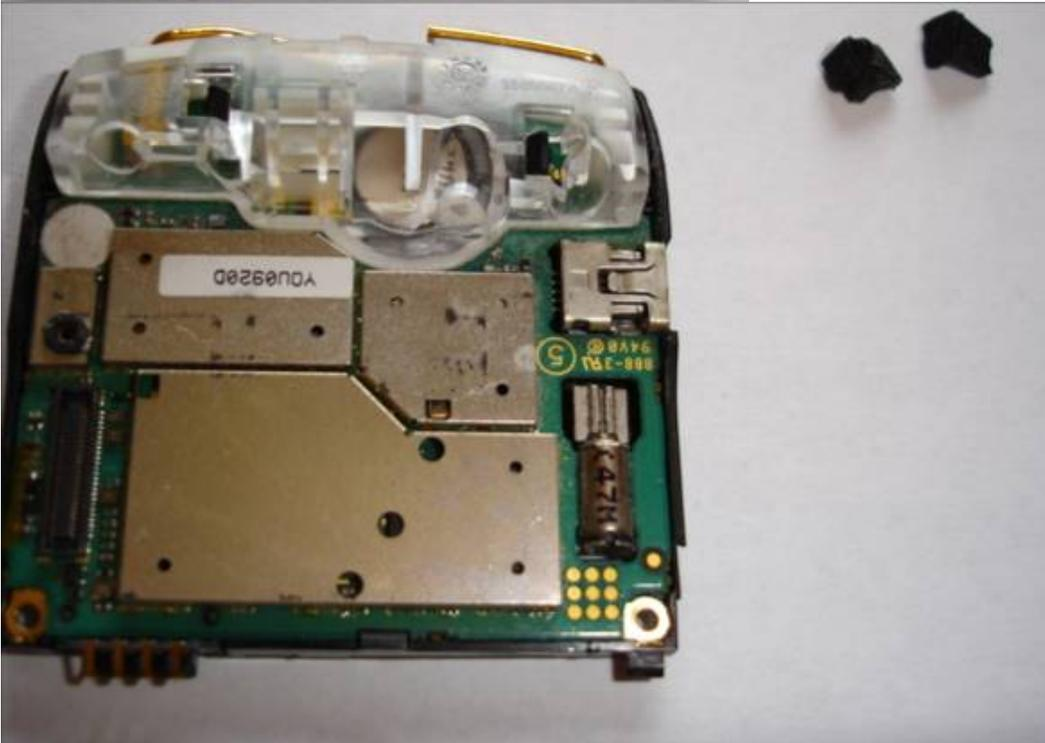
28. Place the screwdriver under the right hand side of the see through plastic covering, CAREFUL DON'T SCRATCH THE PCB! Lift until it clicks and unclips itself. The rest should follow.
