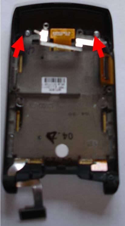
49. Get the screen housing. Place the ribbon through the screen housing.
