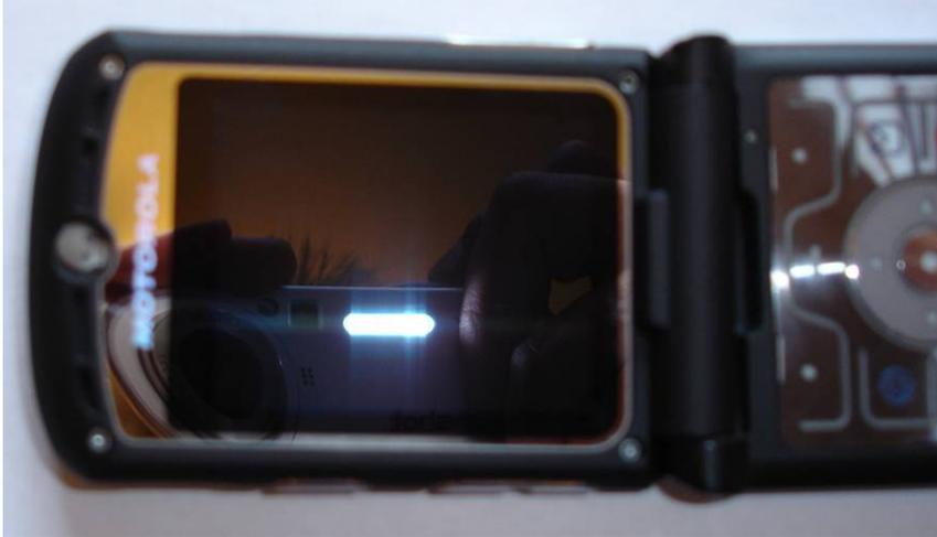
63. Stick the screen down. If your replacing the outer screen put it in now, its easier as the front facia has aligned the screen for you.
