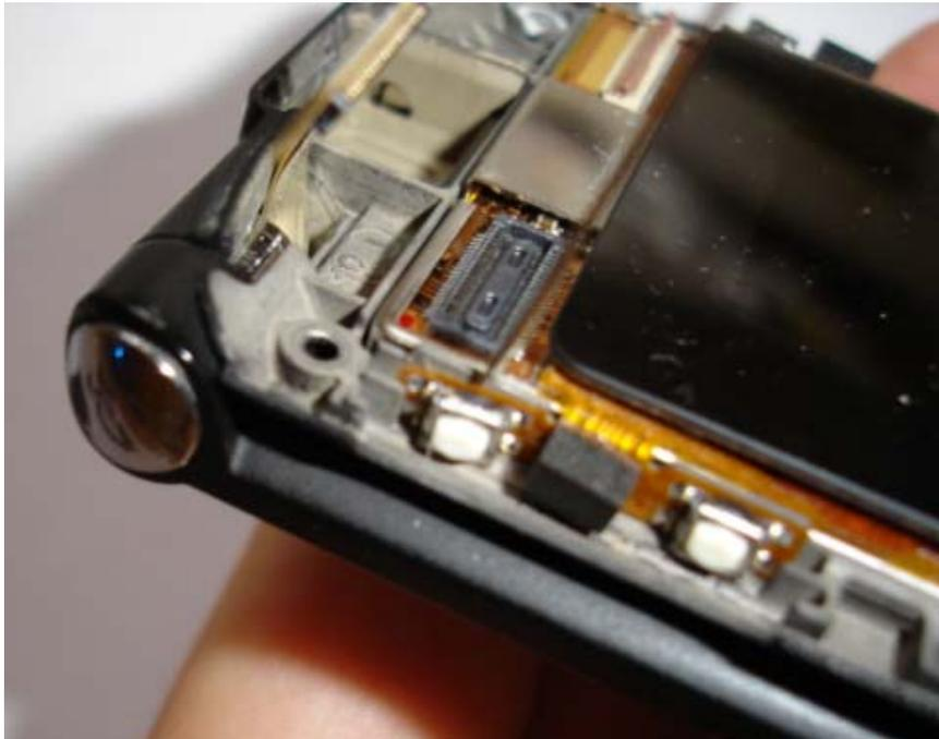
13. Once all of the buttons are unstuck and free from being stuck down. Place the tweezers in the top right of the screen, and slowly start hinging it out. Keep lifting until it comes free.
