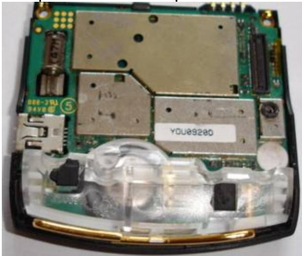
38. Lift up the metal tabs at the bottom of the rear keypad with tweezers.
