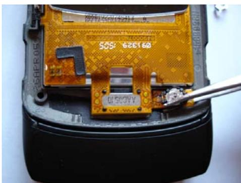
10. Lift the speaker next to it, make sure the sticky pad is still attached. If not peel it off of the housing and stick it to the speaker.
