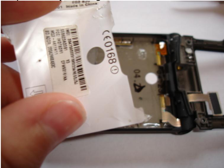
40. Lift up the rest of the metal tabs, make sure that they are all vertical. Then push them one at a time until the keypad comes out.
