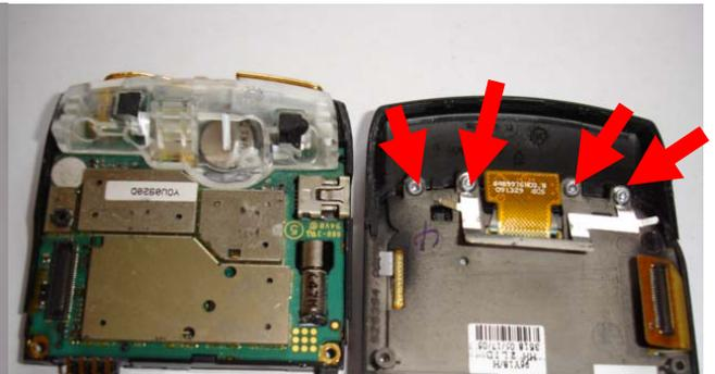
24. You now need to unscrew the 4 screws holding the lower cover on. Use the T5 screwdriver.
