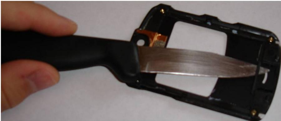
Clean off the glue attached to the frame. With your knife or a sharp craft knife scrape #ing all over were the frame sits. Then use something like Araldite, or super strong bonding adhesive, not just modeling glue. Put some of the bonding agent on the frame and the
