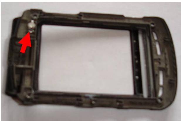
48. Go back to the keypad housing and get the metal part with its screws from step 24. Screw in the two opposite screws first. Make sure the housing is all aligned correctly. Then screw in the middle screws.
