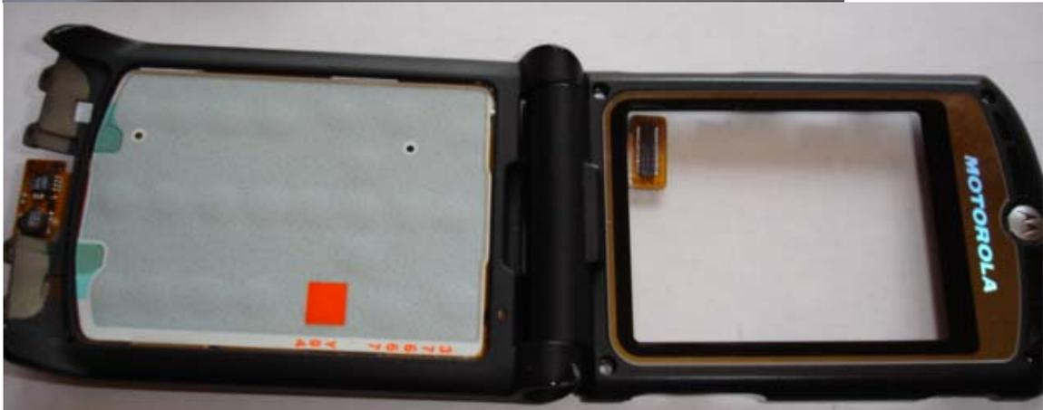
41. Flip the phone over. Push the flipper mechanism as far in as you can and list up the right hand side of the screen. You can lift it out then. **WATCH THE RIBBON ON THE OPPOSITE SIDE, DON'T SEVERE IT!** Unhook the ribbon as soon as you can.
