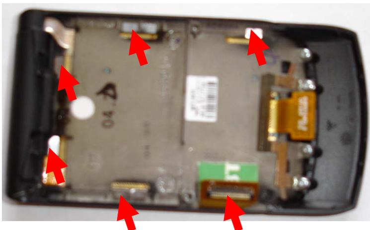
57. Put the white Phone data sticker back down. Use double sided sticky tape or something similar to do this. Then clip in the aerial housing, and screw in. Place the small rubber gromit back in as well.
