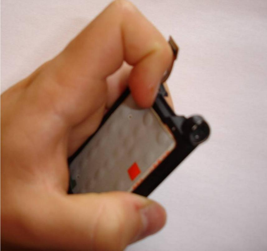
44. Push the tabs through into the new keypad housing and stick down the keypad.
