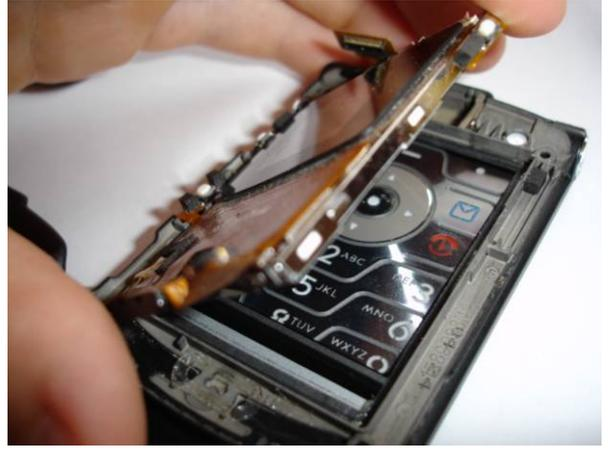
14. Lift the screen out of the Inner screen housing.
