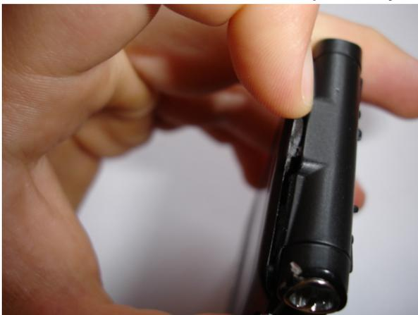
5. Now use the mobile phone opening tool to slide up around the edges of the fascia, work down one side then the other. Then lift the bottom part, it will be quite stiff but keep pulling. Don't be scared you wont damage your phone. Then remove the chrome buttons.
