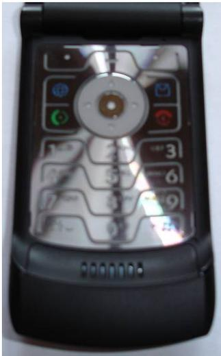
56. Turn the phone over, and while pushing the keypad in as hard as you can bend the metal keypad tabs over.
