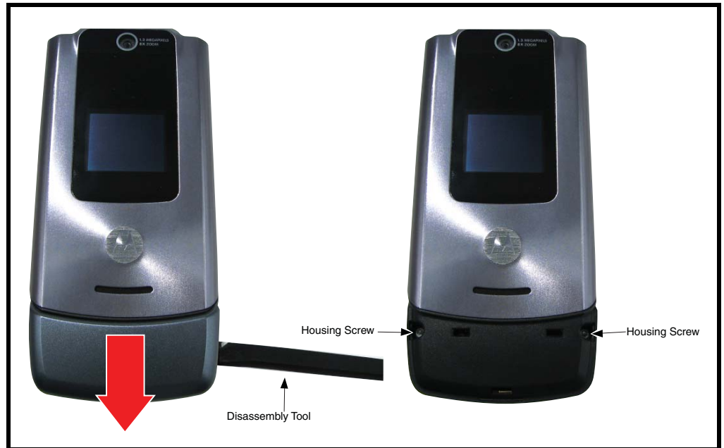
Figure 5. Removing the Rear Housing Latches
