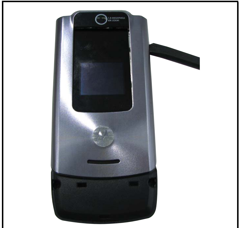
Figure 12. Removing the Flip Assembly Cover
