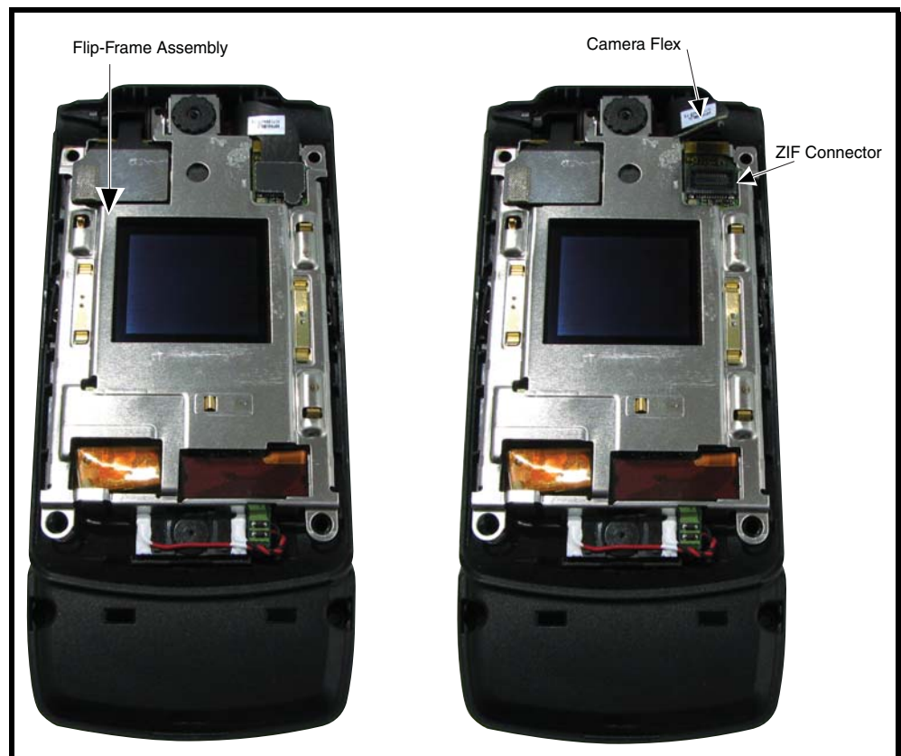
Figure 15. Camera Assembly Removal
