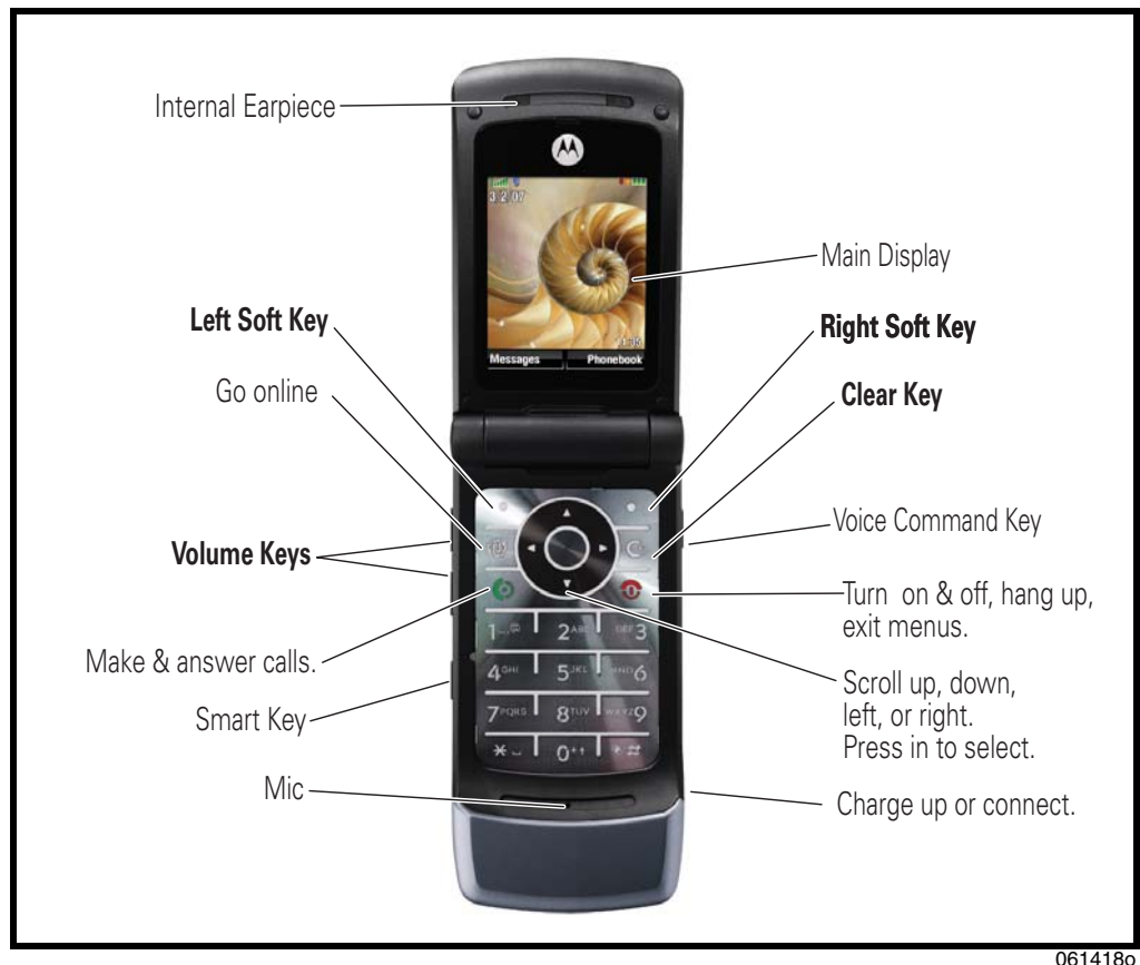
Figure 1. Telephone Controls, indicators, and I/O Connections
