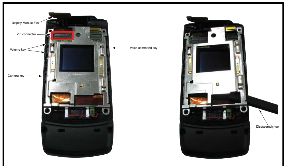
Figure 16. Display Module Assembly Flex Connector
