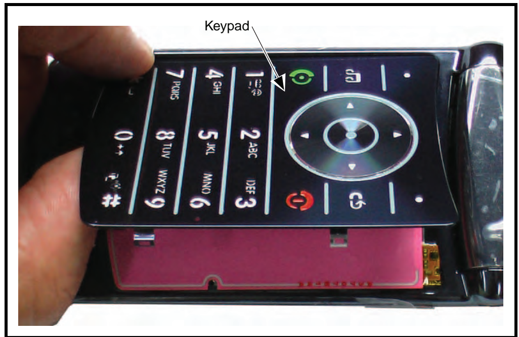
Figure 27. Placing the Keypad into the Front Housing
