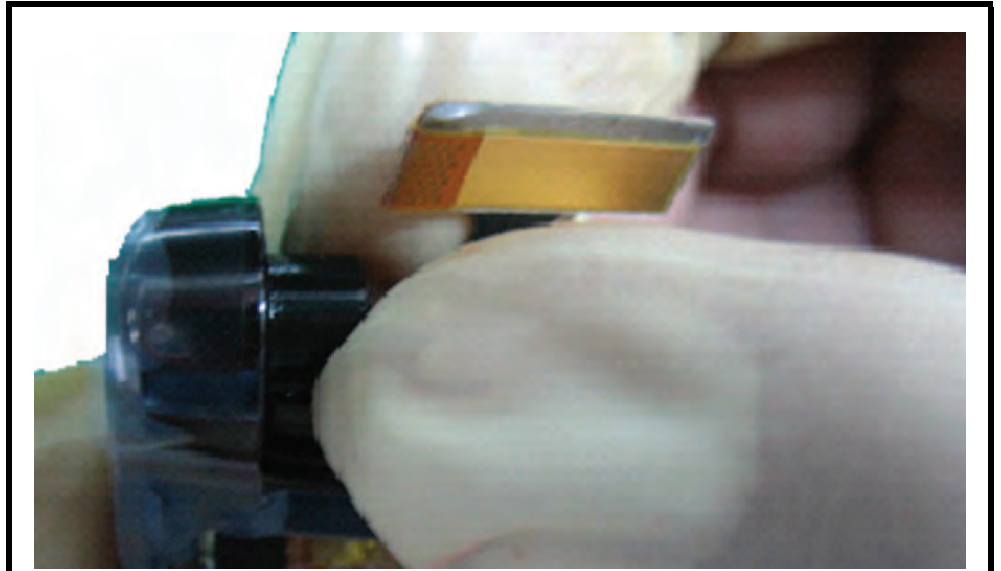
Figure 48. Installing the Housing Sleeve
