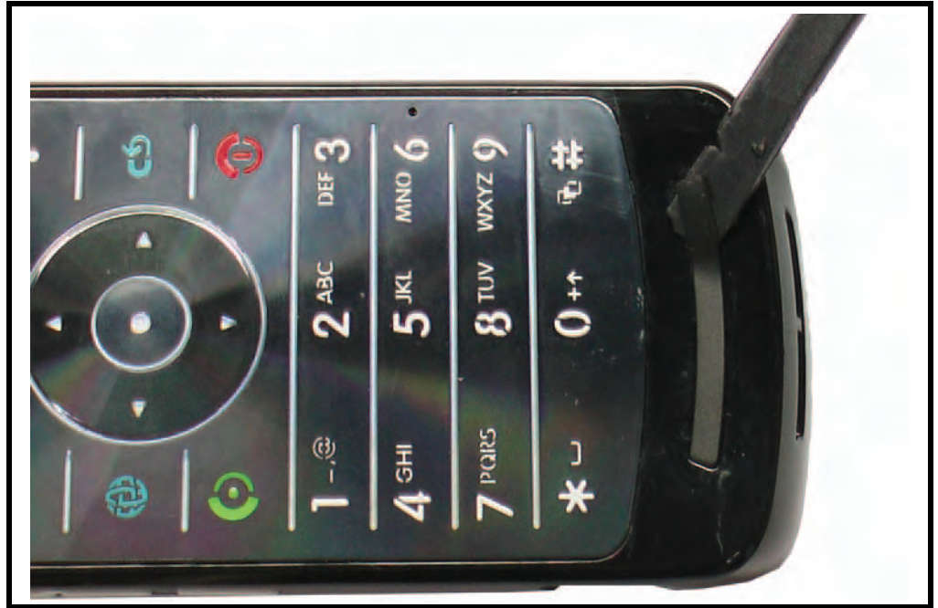
Figure 5. Removing the Bumper
