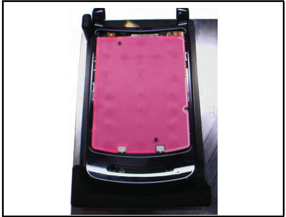
Figure 47. Front Housing Assembly in the Service Fixture
