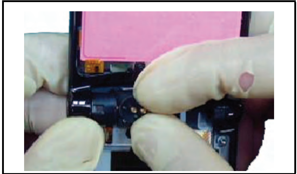
Figure 56. Installing the Vibrator Assembly
