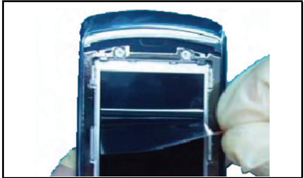
Figure 73. Removing the LCD Liner
