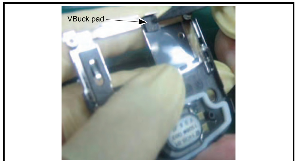
Figure 15. Installing Vbuck Pad in the Rear Housing
