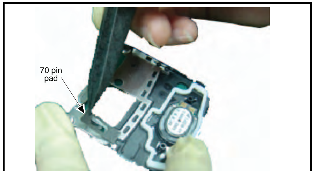
Figure 13. Rear Housing Assembly
