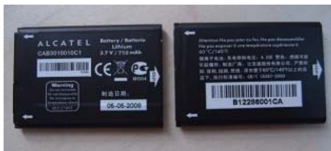
Figure 1.3 - PRESENTATION OF THE BATTERY (Lithium 750 mAh)
