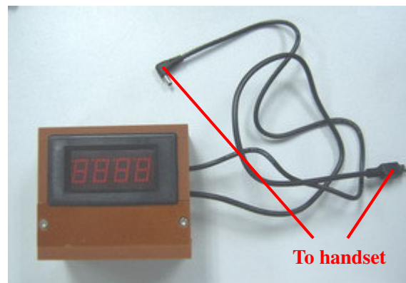
Figure 2.5 – HOW TO CONNECT THE GALVAMOMETRY METER
