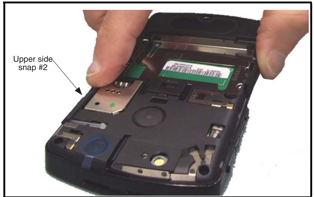
Figure 18. Engaging the Upper Side Snap
