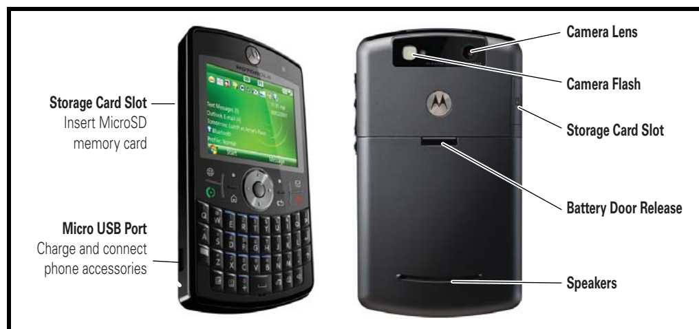
Figure 2. Controls and Indicator Locations, Left and Back
