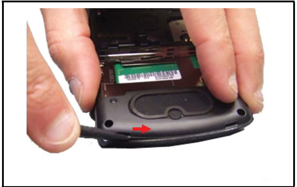
Figure 15. Removing the Rear Housing Snaps
