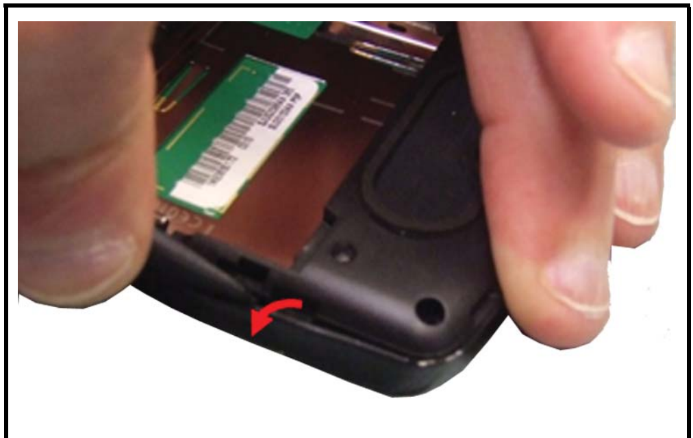
Figure 14. Removing the Rear Housing Snaps
