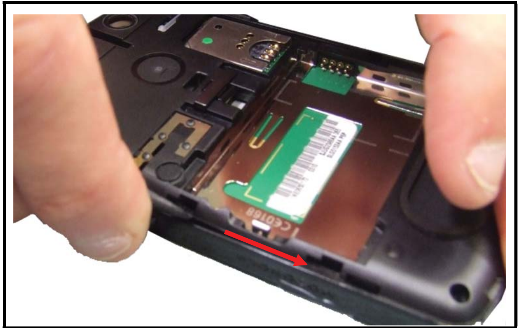
Figure 13. Removing the Rear Housing Snaps
