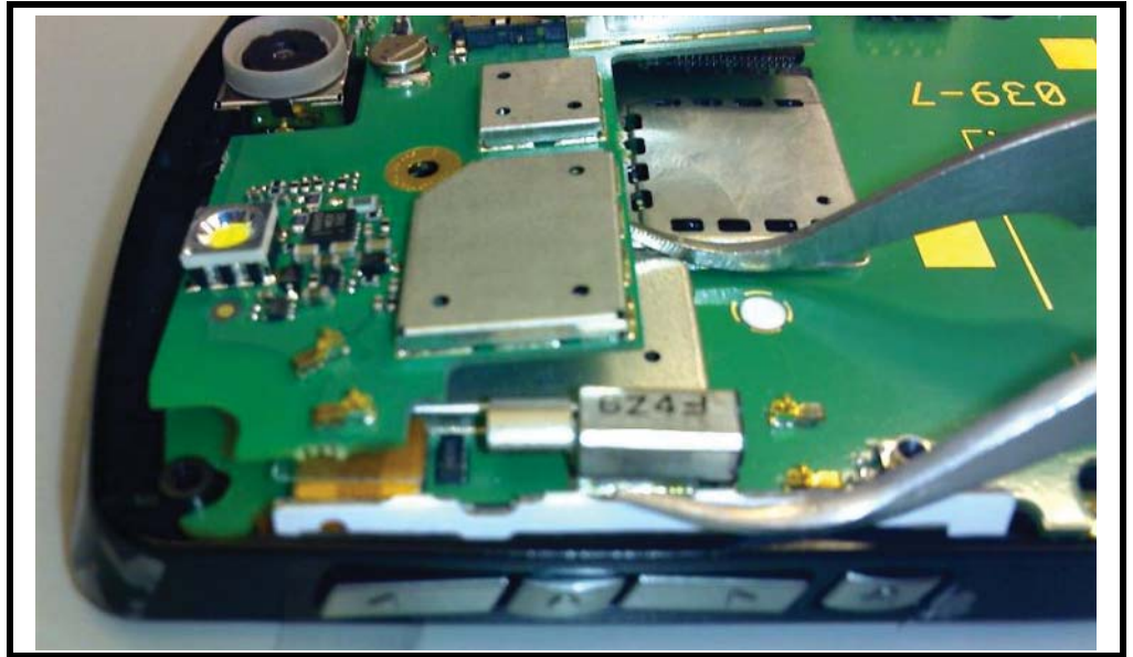
Figure 33. Removing the Daughter Board Assembly
