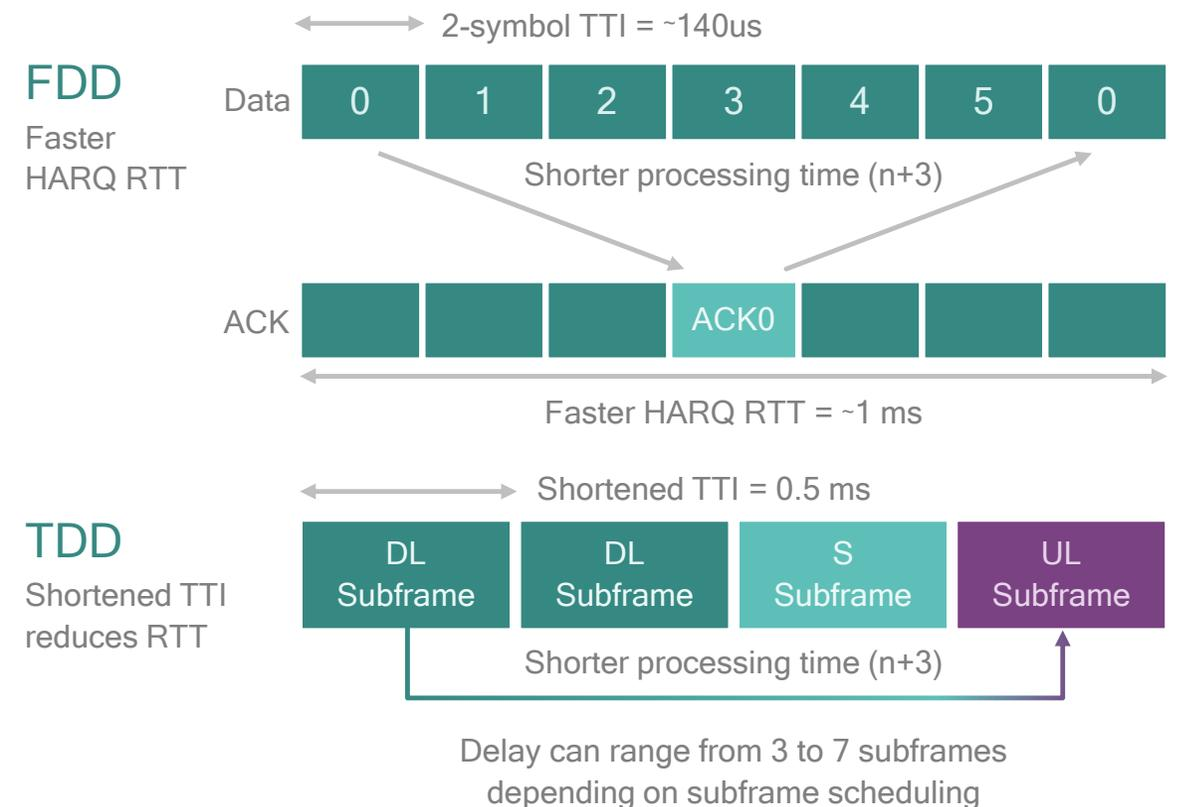
1. Over-the-air latency based on LTE / LTE Advanced HARQ RTT today  $\geq 8$ ms; LTE Advanced Pro = ~1ms based on 2 symbol TTI and n+3 turnaround time; 2. 7-symbol TTI supported for DL/UL TDD; 2/7-symbol TTI supported for DL FDD; 2/4/7-symbol TTI supported for UL FDD
