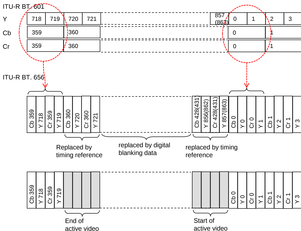
[Fig. 4] Timing Diagram of ITU-R BT601 and ITU-R BT656
