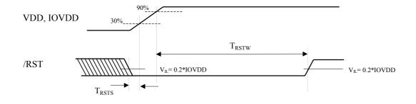
The reset width is defined as the time from the moment VDD or IOVDD has risen to 90%. /RST has to be settled at "L" level at the time VDD or IOVDD has risen to 30%.
