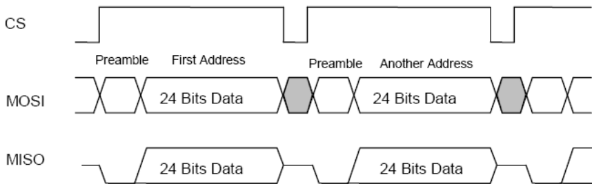
Figure 6. SPI Transfer Protocol Multiple Read/Write Access
