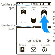
To move a button or scroll through a screen, just touch the display and slide the button or icons
