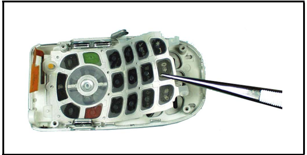
Figure 12. Removing the Keypad, Volume/Smart, and Voice Buttons
