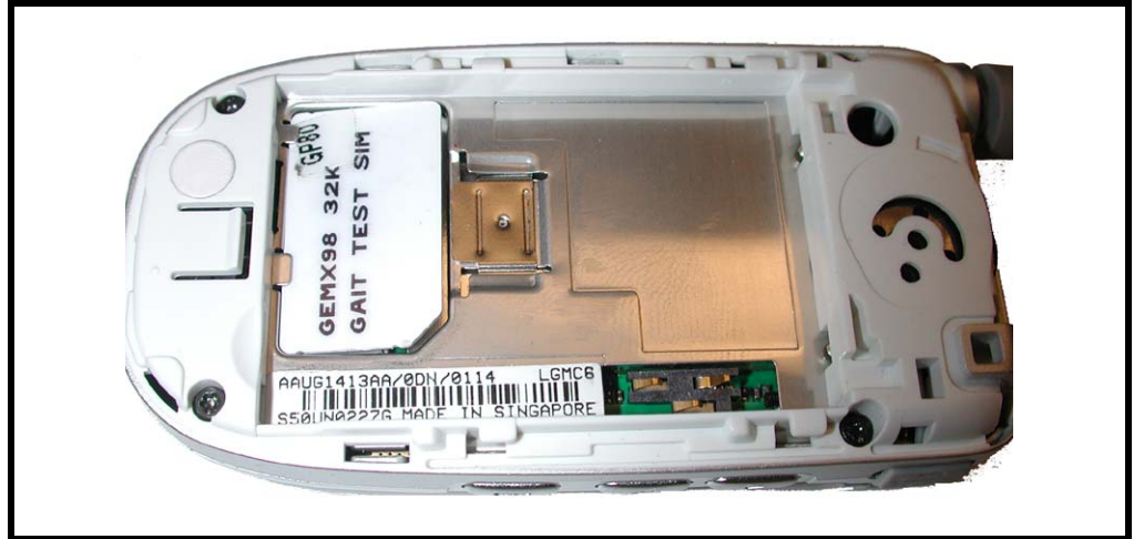
Figure 3. Removing the SIM
