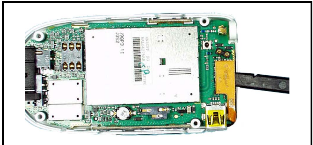
Figure 9. Disconnecting the flex from the transceiver board
