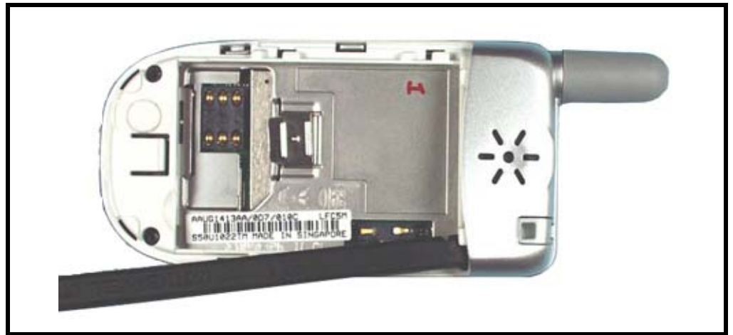
Figure 4. Removing the Polyphonic Speaker Cover
