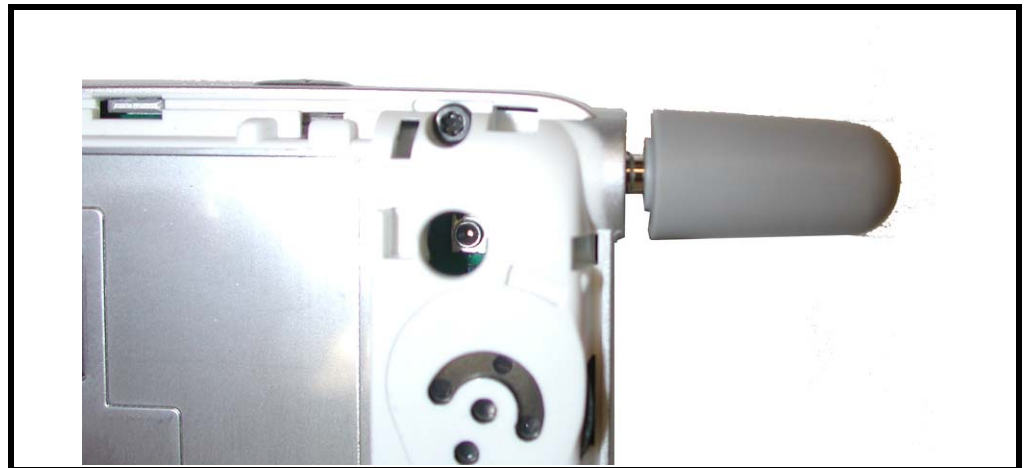
Figure 5. Removing the Antenna
